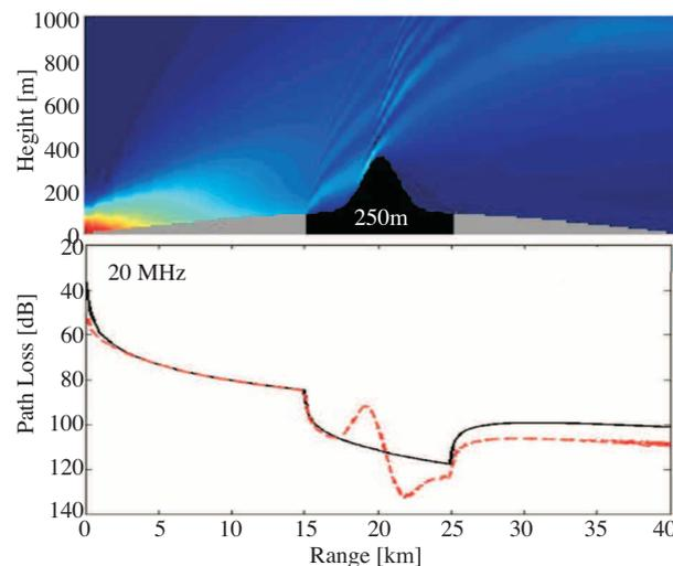
**Figure 3.** A typical mixed-path propagation scenario and longitudinal signal variation.
