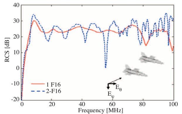
**Figure 5.** Two F-16 flying side-by-side and their RCS vs. frequency curves.
