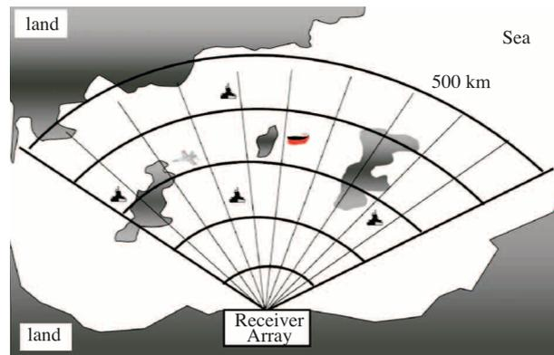
**Figure 2.** A typical HFSWR scenario: Range, cross-range resolution and radar cells [4].
