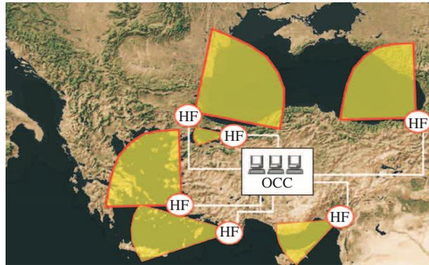
**Figure 1.** A typical HFSWR based IMS system.
