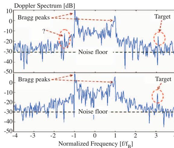
**Figure 6.** Two Doppler spectra showing total HFSWR echoes. The spectra contain noise, clutter and target (SNR=13 dB, CNR=30 dB, Noise floor is set to -30 dB).
