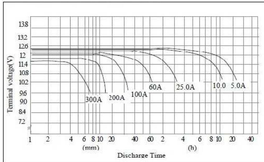
**Fig. 3** Discharge curve of marine type gel batteries [1]
