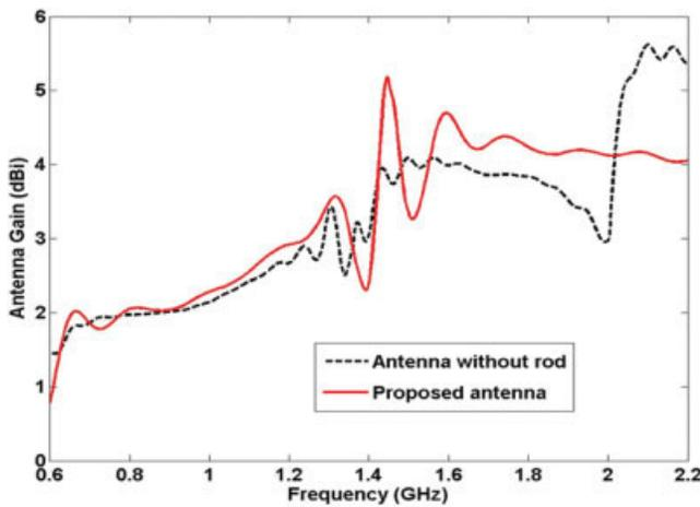
**Figure 6** Antenna gain of the proposed antenna and the antenna without rod. [Color figure can be viewed in the online issue, which is available at [www.interscience.wiley.com](http://www.interscience.wiley.com)]
