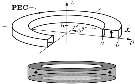
Figure 1: Rectangular cross section ring resonator
