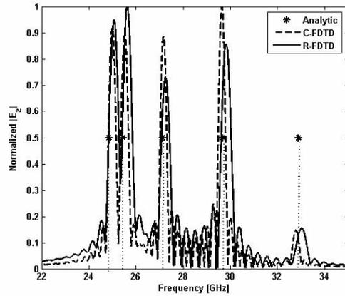
Figure 4: Resonance frequencies obtained via C-FDTD (dashed), R-FDTD with fine grid (solid) and analytic solution (symbol)
