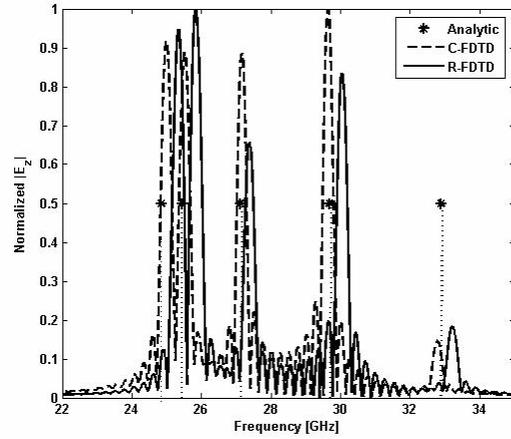
Figure 3: Resonance frequencies obtained via C-FDTD (dashed), R-FDTD with coarse grid (solid) and analytic solution (symbol)
