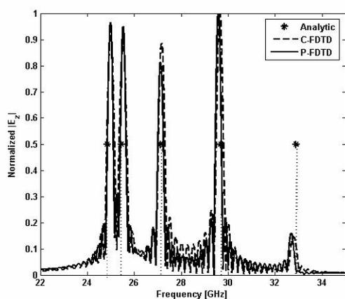
Figure 5: Resonance frequencies obtained via C-FDTD (dashed), P-FDTD (solid) and analytic solution (symbol)
