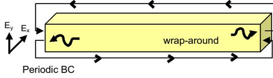
Figure 2: Rectangular cross section waveguide with PBC applied at input and output ports
